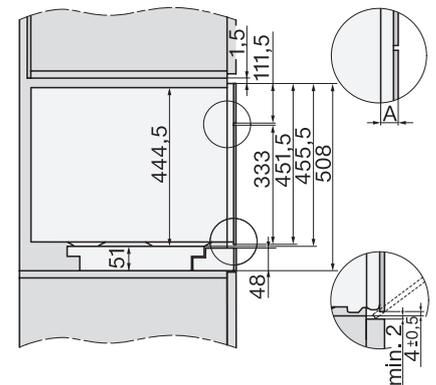
side view DG7xxx-55 compensating cover at the bottom, installation drawings, CH
