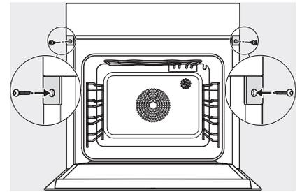
screw joint DGC XXL, installation drawing
