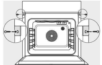
screw joint DGC XXL, installation drawing
