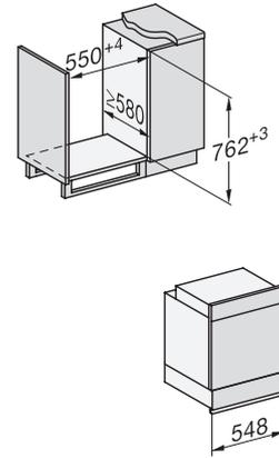
built-in H7000-55 build-under, installation drawing
